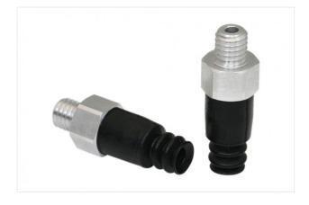
Size: 5 Suction cup material: Nitrile rubber NBR Material hardness: 55 °Sh Nipple material: Aluminium Vacuum connection: M5-M Number of folds: 2.5
