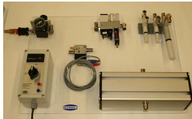
The electromagnetic valve (EMV) is activated by the evacuation time counter. Please connect the plugs of each color (correct polarity). The electromagnetic valve is closed in passive state (NC). By moving the switch of the evacuation time counter (“valve on”) the EMV will be opened and compressed-air will channel to the basic ejectors.
