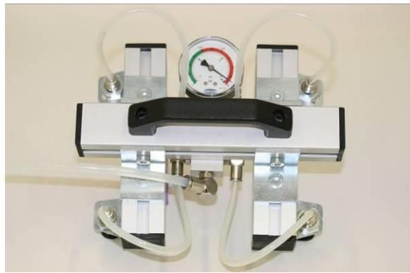
The present suction pads (FSGA 20.0 NBR) can be attached via pinning on the nipples. You will also need a reduction nipple for further exercises for the suction pads FSGA 32 HT1 and FSGA 33 HT1 to reduce the connection of the suction pad from G1/4-AG to G1/8-AG (see figure).
