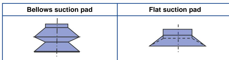
Flat suction pads are particularly suitable for handling of objects with flat or only slightly curved surfaces. For example sheet metal boards, cardboards, glass panels, plastic parts or wooden plates.
