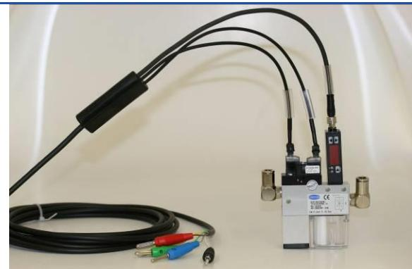
Affiliate a choke valve in-between the volume storage and the gripper system as shown in the picture below. An artificial leakage can be simulated by the help of the choke valve.
