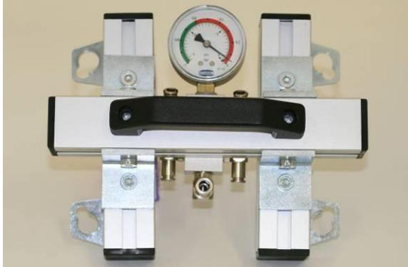
A photograph showing the gripper system in its original state. It consists of a central black actuator plate mounted on a silver-colored holder. On either side of the actuator are two white rectangular pads. A pressure gauge is mounted above the gripper, connected by a tube. The entire assembly is mounted on a light-colored surface. |
