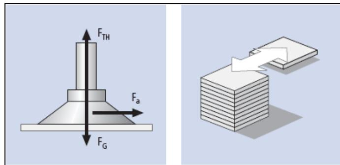
**Load case III – Suction pads vertical, force vertical**
