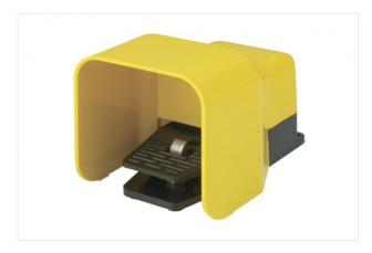
Nominal size: 7 mm Function: 3/2-way valve Thread G1: G1/4-F with: Detent
