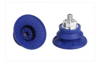
Size: 60 Suction cup material: Nitrile rubber NBR Material hardness: 60 °Sh Vacuum connection: M10-M Nipple material: Steel Number of folds: 1.5
