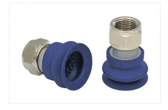
Size: 30 Suction cup material: Nitrile rubber NBR Material hardness: 60 °Sh Vacuum connection: G3/8-F Nipple material: Brass, nickel-plated Number of folds: 1.5
