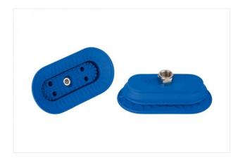
Dimensions (LxB): 140 x 70 mm Suction cup material: High temp material HT1 Material hardness: 60 °Sh Nipple material: Brass, nickel-plated Vacuum connection: G3/8-F Number of folds: 1.5
