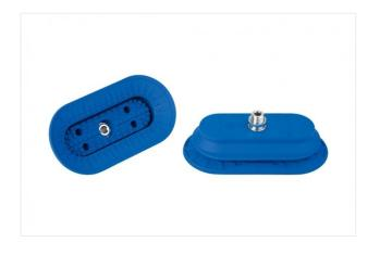
Dimensions (LxB): 140 x 70 mm Suction cup material: High temp material HT1 Material hardness: 60 °Sh Nipple material: Aluminium Vacuum connection: G1/4-M Number of folds: 1.5
