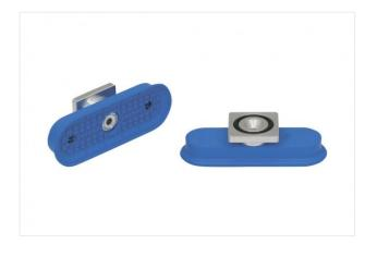
Dimensions (LxB): 90 x 30 mm Suction cup material: Nitrile rubber NBR Material hardness: 45 °Sh Nipple material: Aluminium Vacuum connection: Rectangular adapter
