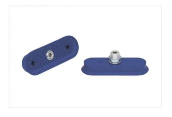
Dimensions (LxB): 90 x 30 mm Suction cup material: Nitrile rubber NBR Material hardness: 60 °Sh Nipple material: Aluminium Vacuum connection: G1/4-M
