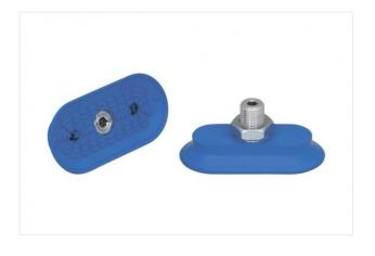
Dimensions (LxB): 80 x 40 mm Suction cup material: Nitrile rubber NBR Material hardness: 45 °Sh Nipple material: Aluminium Vacuum connection: M14x1.5-M
