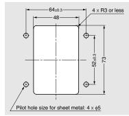
\*The dimensional tolerance for installation holes drilled in sheet metal is  $\pm 0.3$ .
