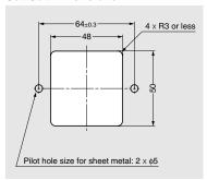
\*The dimensional tolerance for installation holes drilled in sheet metal is ±0.3.
