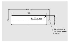
\*The dimensional tolerance for installation holes drilled in sheet metal is  $\pm 0.3$ .
