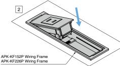
To remove the product, push in the catch of the bracket on the back. See the instruction manual for details.
