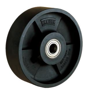
Untyred wheels can carry high loads with low rolling resistance when used on a hard surface such as flat steel. On softer surfaces, such as concrete or tarmac, the surface is likely to be worn or indented by the use of an untyred wheel. Untyred wheels are noisier in operation than tyred wheels, but noise is unlikely to be a problem at walking speeds.
