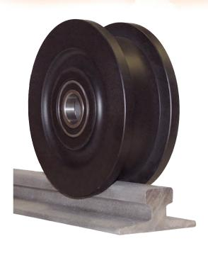
Cast iron rail wheels are the most economic for light to medium duty, but they have a limited service life when compared to steel wheels, and are unsuitable for high rotational speeds or where substantial shock loads are to be withstood.
