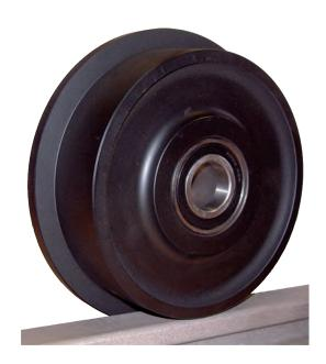
Cast iron rail wheels are the most economic for light to medium duty, but they have a limited service life when compared to steel wheels, and are unsuitable for high rotational speeds or where substantial shock loads are to be withstood.
