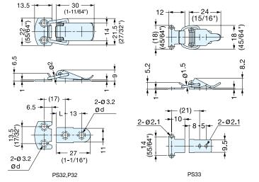
\*Dimension shown is in case of clamping force "0".
