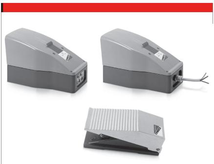
The pedals can be supplied in either a pneumatic or electrical foot operated version. The pneumatic type is available with a 5/2 valve and G1/4 front ports, which allow the fittings and silencers to be assembled conveniently on the front face. A 3/2 operation can be obtained by closing an outlet port.
