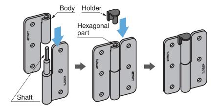
Insert the body into axis, and then insert the holder into the hexagonal part of axis to generate torque.
